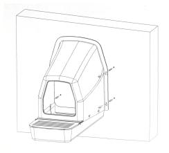
Use nesting box as template to mark and drill holes in the wall. Insert plastic screw anchor into each hole. Use screws to attach the nesting box to the wall
