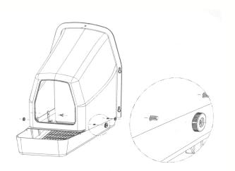
One at a time, push the bolts through the holes from the outside. Attach white nut
