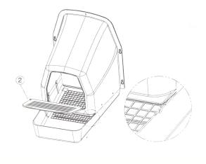
Attach lid (2) to basket as shown. Press down until the lid snaps into the grooved indents in the basket
